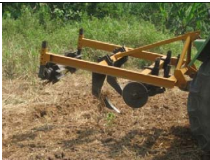
Ndume ripper used to create double rip lines for the pilot trial.
