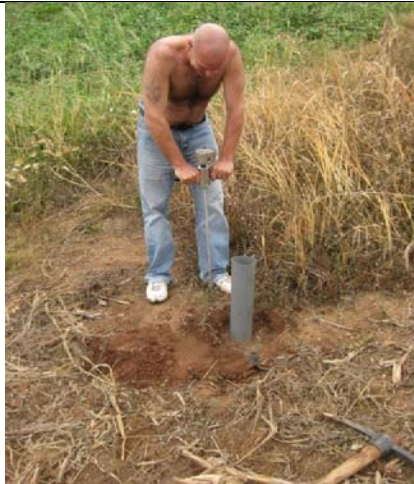
Penetrometer and water infiltration tests were part of a survey aimed at understanding soil compaction and sub-soil drainage patterns.
