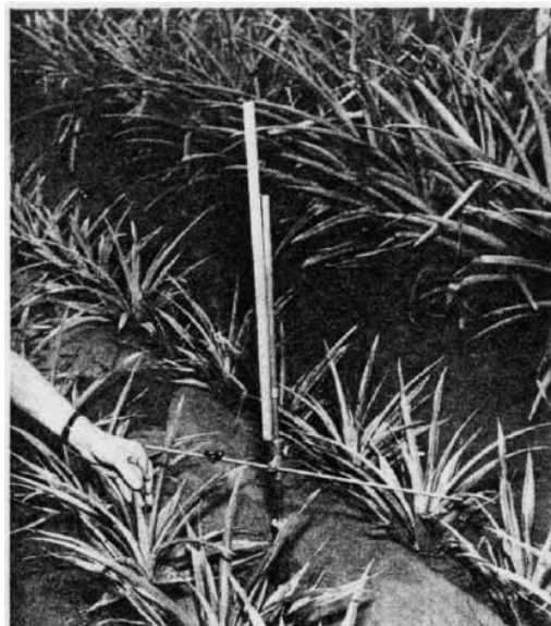
Figure 2. Leaf elongation meter, a portable instrument for measuring leaf elongation. A metal pipe is driven into the ground as a permanent bench-mark. The meter is placed on the pipe and the height of a heart leaf of 7 or 8 plants is measured at each location.
