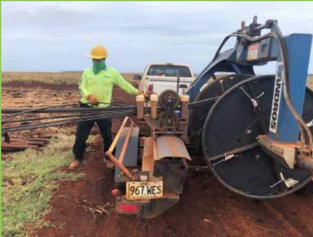
Figure 5. Drip tube retrieval machine.
