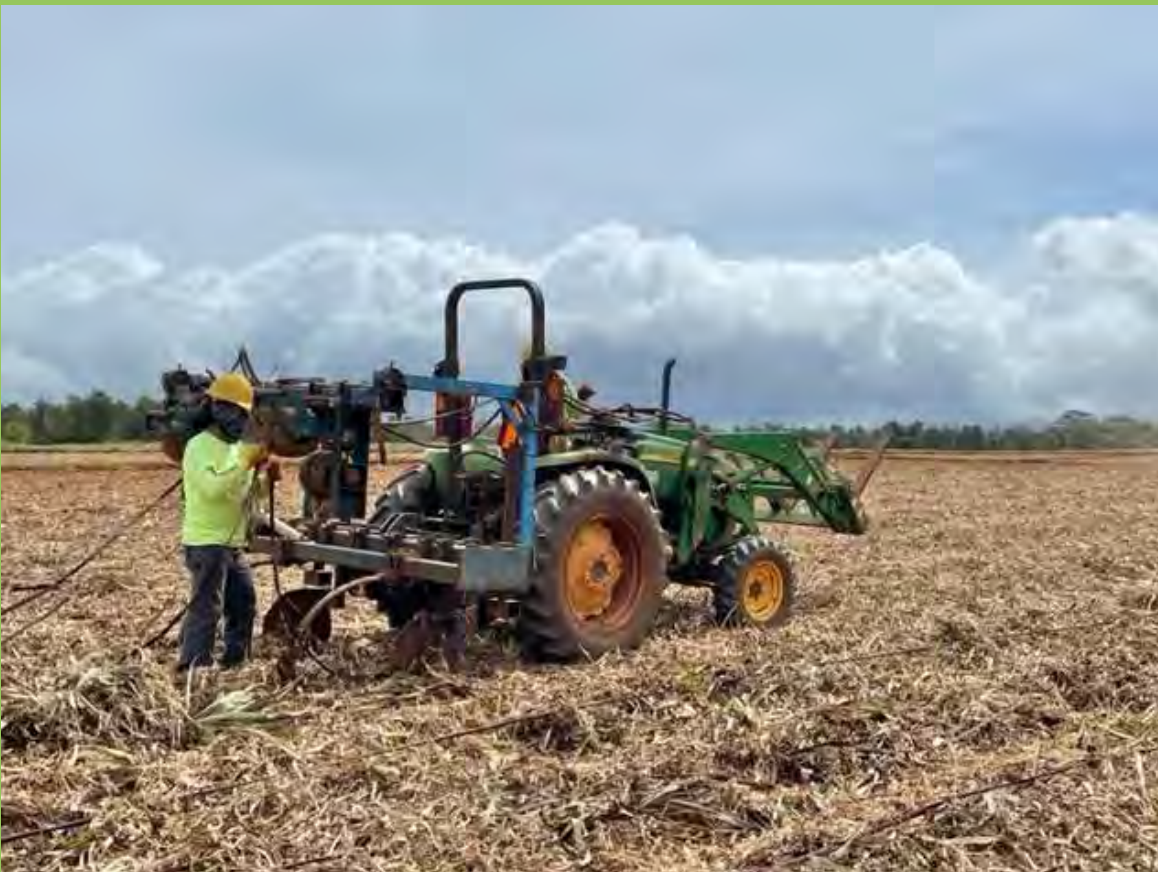
Figure 3. Lifting/extracting the tubing out of the ground.
