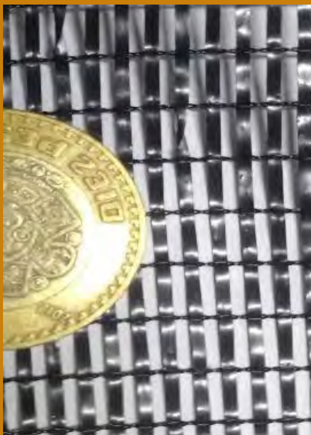
Figure 5. In at least five works of the Inifap-Papaloapan, types of MSP were evaluated (photos from left to right): A) Rashel flat woven ribbon; B) Monofilament round thread, and C) Hybrid extended flat ribbon crossed with round thread. Subsequently, degrees of shade were studied (35, 45, 50 and 65%) of MSP Rashel vs MSP Monofilament, but only in two fruit harvest seasons: Late Winter and Mid-Autumn. The MSPs were installed one to two months before flowering forcing; the control was the regional fruit protection practice of tying the leaves with plastic raffia over the fruit. It was concluded that the black Hybrid MSP (C) is the most suitable one due to its resistance, ease of handling and cost, especially in high-density plantings in first and second ratoon cycles, where the protection of the fruits with conventional methods is impractical and unaffordable. 50% shading turned out to be more convenient and useful for the whole year. In spring-summer time, a period considered more critical for medium to large fruits, harvested at intermediate to advanced maturity degrees (2, 3 and 4), shading up to 65% may be required. However, in plantations with fruits destined for the fresh export market (with densities of 60 to 70,000 plants/ha), this high degree of shade may reduce fruit weight by 5% when harvested in autumn and winter, what is considered to be a small inconvenience, when compared to the advantages achieved with the MSP in relation to the other regional methods.
