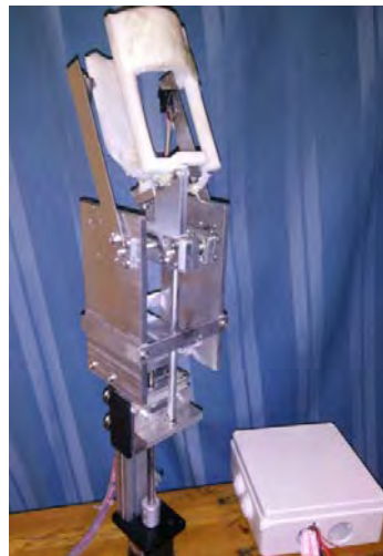
Figure 4. The second end-effector for harvesting robot.
