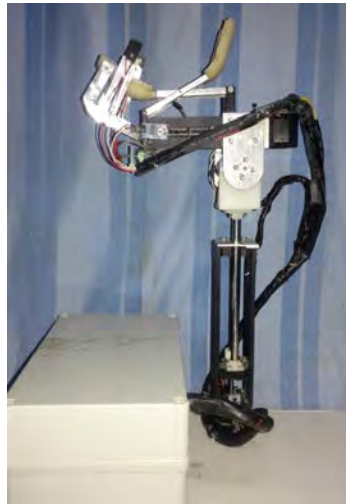
Figure 3. The first end-effector for harvesting robot.
