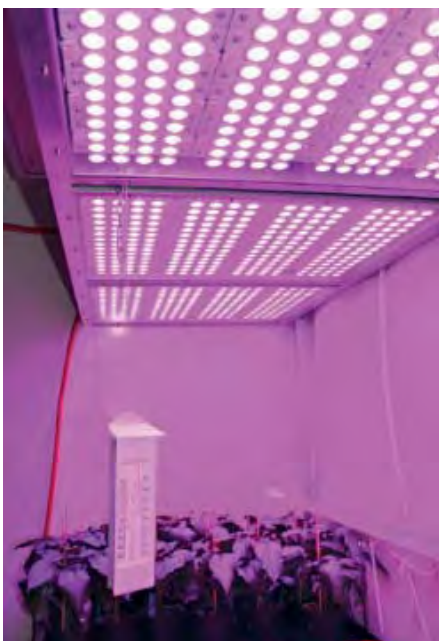
Figure 6. Growing sweet pepper in a plant growth unit employing the latest LED technology. Photo: G. Noga.
