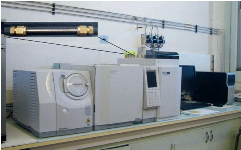
Figure 3. The quantity and quality of volatiles released by plants may indicate the presence and type of stress, as well as the plant's capacity to cope with the stress. They can be measured by sampling the headspace air around plant organs on cartridges containing an adsorbent, which are subsequently analyzed by thermal desorption/injection unit coupled to a gas chromatograph with mass spectrometer.
