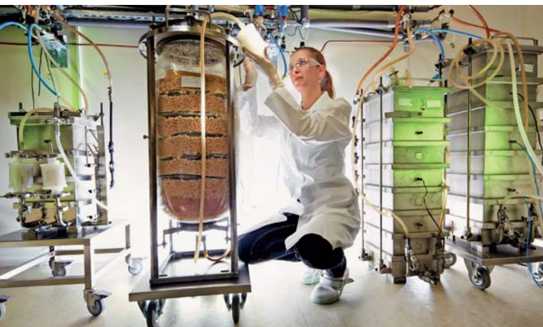
• Searching for new biological compounds: Bayer CropScience employee Melanie Röpcke tests the growth of fungi in a fermenter in Wismar, Germany. •••••
