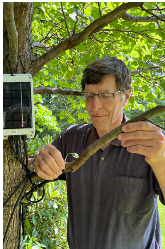
► Alan Lakso checking the installation of a microtensiometer in a tree (2024).
