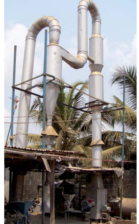
Modern flash-dryer equipment in cassava processing plants in Lagos, Nigeria.
