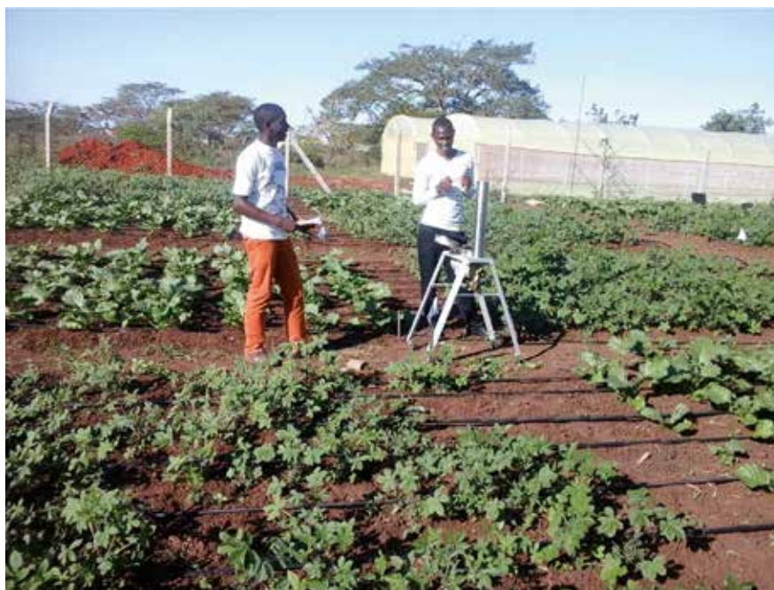
› Undergraduate horticulture students from Kenyatta University of Agriculture and Technology collecting leaf water potential data using a Scholander pressure bomb. Photo: Osia Odula (HORTINLEA PROJECT, 2015).
